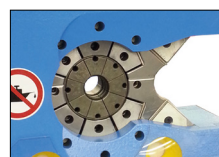
Constant axial centre when crimping jaws are closed.
