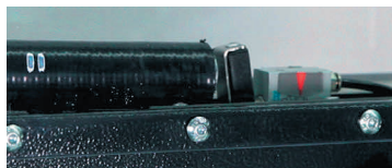
UNIFLEX insert – marking tool (ferrule position marking increases productivity and improves safety in hose sizes up to 2".
