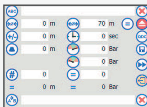
Input of press dimension, correction values, hold time, opening diameter, preselection counter and press dies (automatic).
